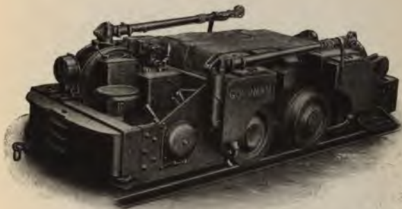
Crab Reel Driven by Independent Motor
